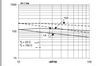
Fig.9. Modulator maximum  $t_{rr}$  measured to 25% of  $I_{rm}$ ;  $T_j = 25^{\circ}\text{C}$  and 150  $^{\circ}\text{C}$
